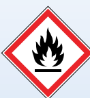
GHS 02 Flammable Self-reactive Pyrophoric liquids & solids Self-heating reactive Emit flammable gases Organic Peroxides
